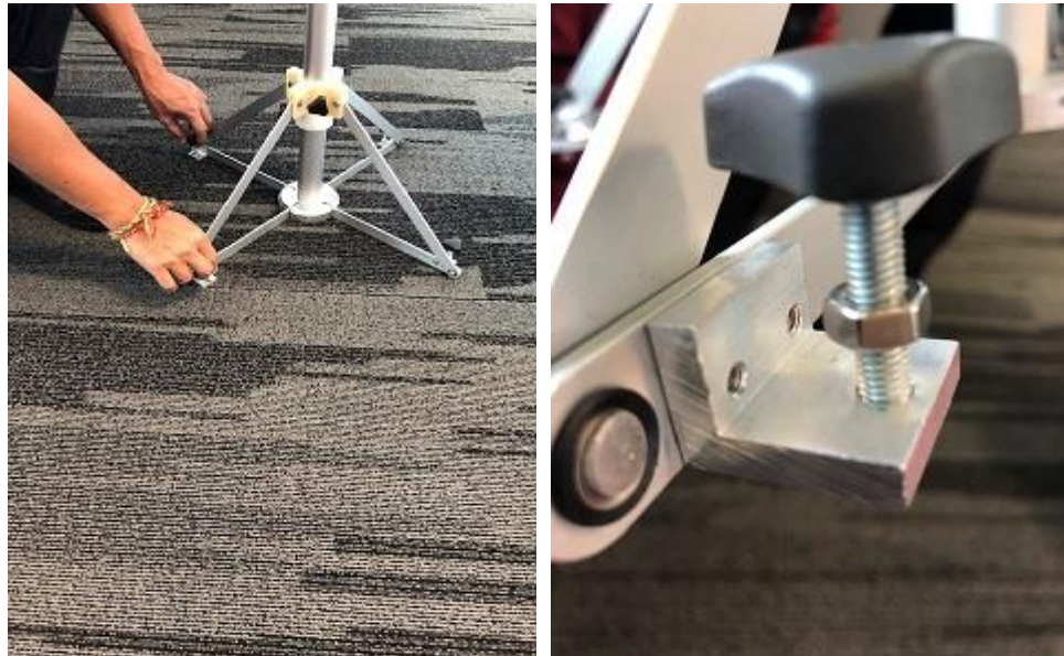
Further adjustments can be made to lock the screw to the floor
