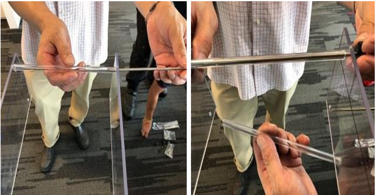
Inserting long screws to hold the acrylic together
