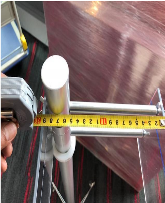
19cm distance between each acrylic near the pole
